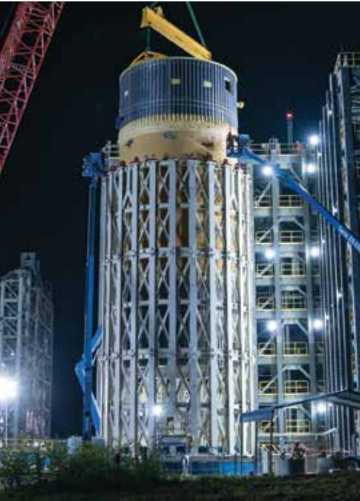
NASA conducts structural tests on the Space Launch System. Photo courtesy of Boeing
